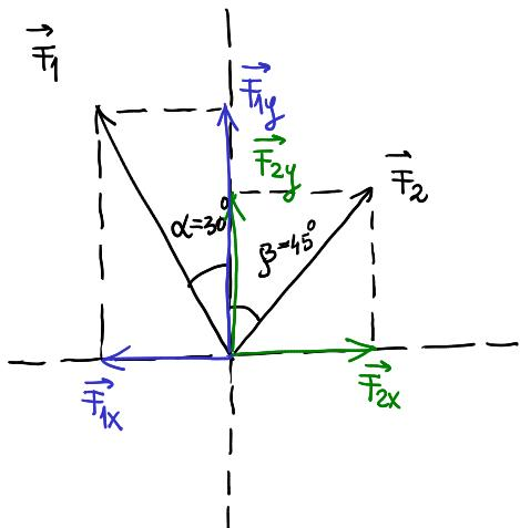
$$\begin{aligned}\vec{F}_{1x} &= \vec{F}_1 \sin \alpha \\ \vec{F}_{1y} &= \vec{F}_1 \cos \alpha \\ \vec{F}_{2x} &= \vec{F}_2 \sin \beta \\ \vec{F}_{2y} &= \vec{F}_2 \cos \beta\end{aligned}$$
