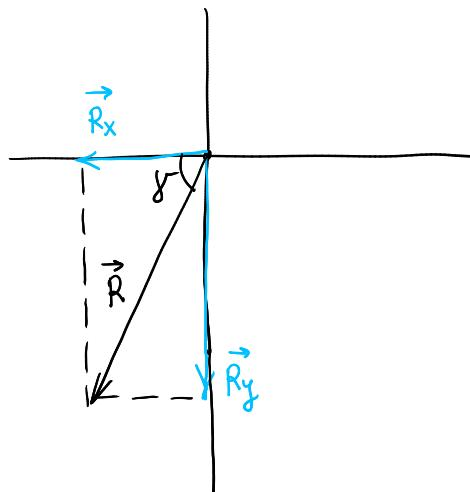
$$\begin{aligned}\vec{R} &= \vec{R}_x + \vec{R}_y \\ R &= \sqrt{R_x^2 + R_y^2}\end{aligned}$$
